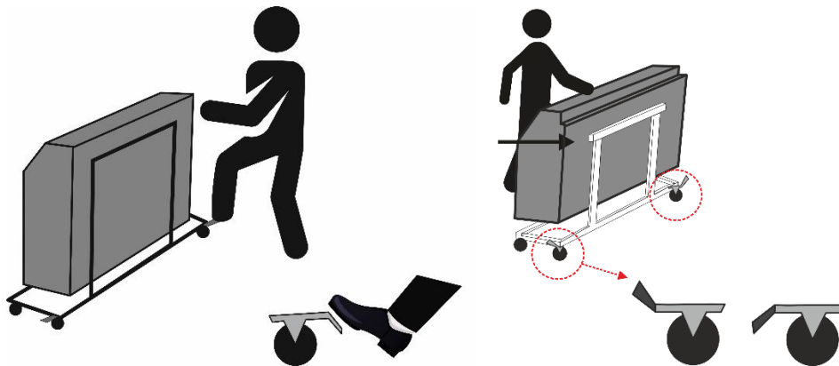
Picture: After moving Athmoss on the mobile stand to the application site, secure the wheel brake (locking). The wheel brake is locked when the brake lever is down. The wheel brake is released when the lever is up.
