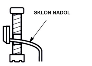
Proper installation of condense hose
